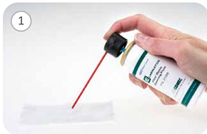
1 Spray a small amount of cleaning solvent on an optical grade wipe
