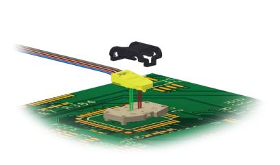
PRIZM® LightTurn® Connector with PRIZM® LightTurn® MOI in Embedded Module Application
